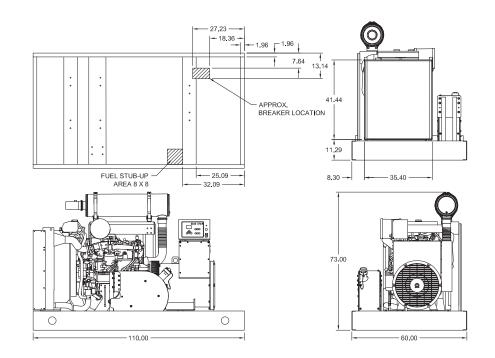
Drawings based on standard open power 480 volt standby generator. Lengths may vary with other voltages. Subject to change without notice. Sound data as measured at 23 feet (7 meters) in accordance with ISO 8528-10 at standby rating.
